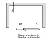
Heat Source: 500mm clearance from an external heat source is required in order to protect the oven control components and allow access to the service panel. For clearances under 500mm, it is mandatory for Stoddart heat shields to be fitted while
